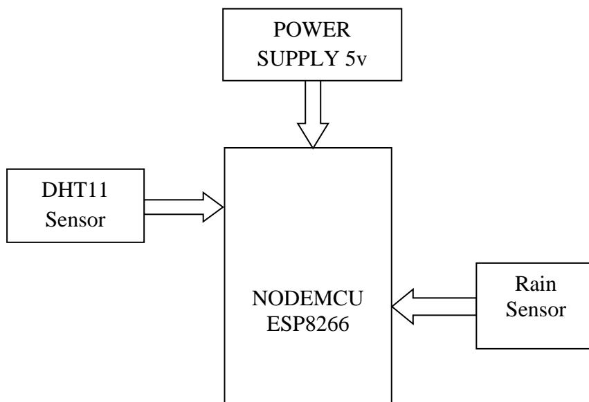
In above block diagram It consists of Rain Sensor, DHT11 Sensor, the Nodemcu and the all sensors are used to detect the Humidity, Temperature, Rainfall in each bin, and it will send this information to the Nodemcu, which acts as the system controller. In the case where the bins are already full or almost full, then it will generate a output of the BYNK app for mobile.
